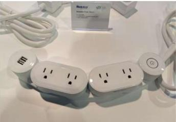
The 3-in-1 power strip is integrated with 3 methods to charge, AC socket charging, USB charging and wireless charging. It is equipped with 2 US sockets and 2 USB ports on the side panels, and features a 10W wireless charger on the top to charge Qi-certified devices such as iPhones and Samsung smart phones.
