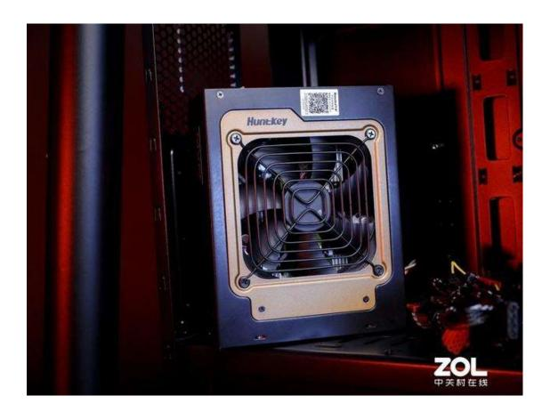
First of all, the power supply must be able to meet the needs of the platform. A 400W or 500W power supply can't meet the needs. But if it is a 800W power supply, will definitely support for the dual-card platform, not to mention the single-card flagship platform.
