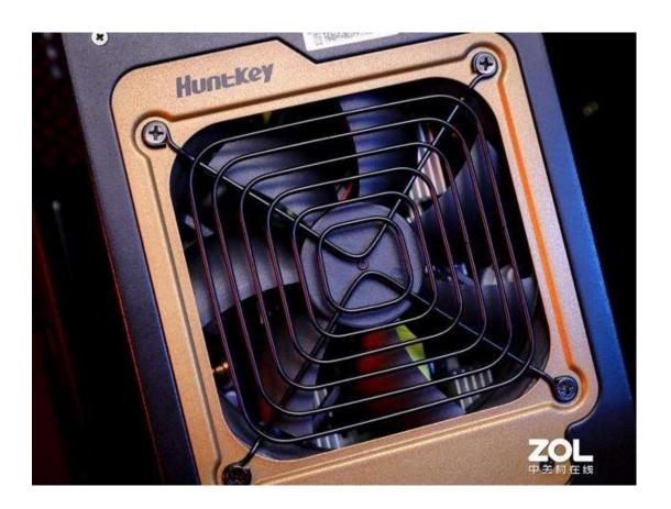
Another point that gamers usually pay attention to is noise. We know that the noise is generated when cooling system works. The higher conversion efficiency the less heat generate while the power supply work. With the efficient cooling system, the noise is much less than the ordinary power supply.
