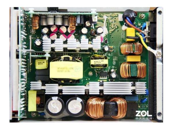
Besides power-saving, the internal design is also essential. Engineers usually have an overall consideration when they develop a high-end power supply. The active PFC + LLC resonant + DC toDC architecture is a common and a mature design. It has efficient and stable advantages .
